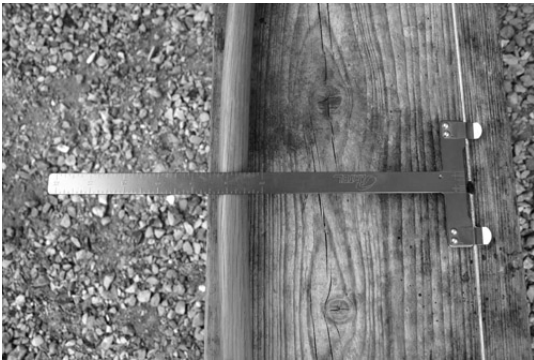
Measuring brace height using a bow square.
